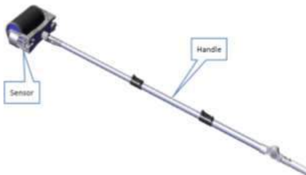
Figure 2. Sub-Surface Profiler (SSP) Components (Reutechmining, 2017)
