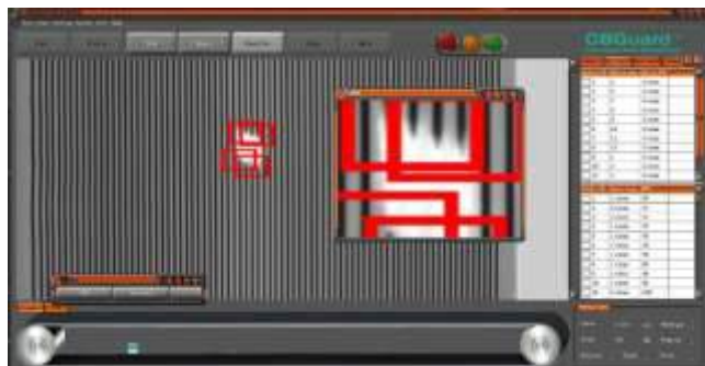
Figure 3. Automatic marks of belt failures
