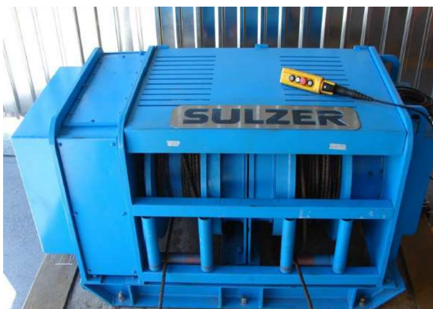
Figure 4. Sulzer automatic remote control winch
