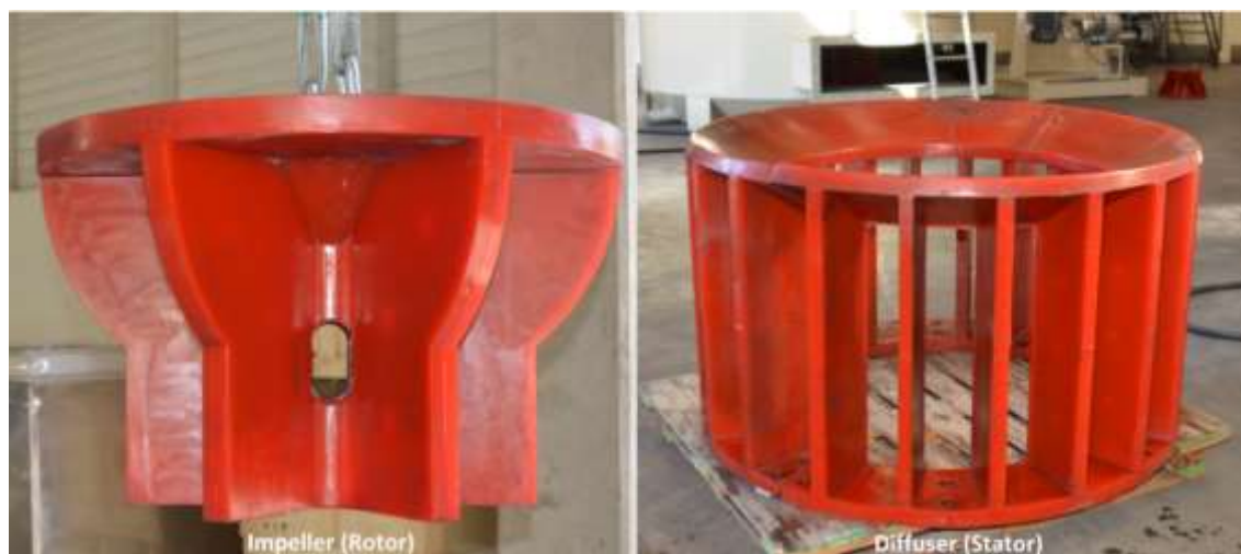
Figure 4: The impeller and stator of the TK Cells (Courtesy of Tüfekçiöğlü)
