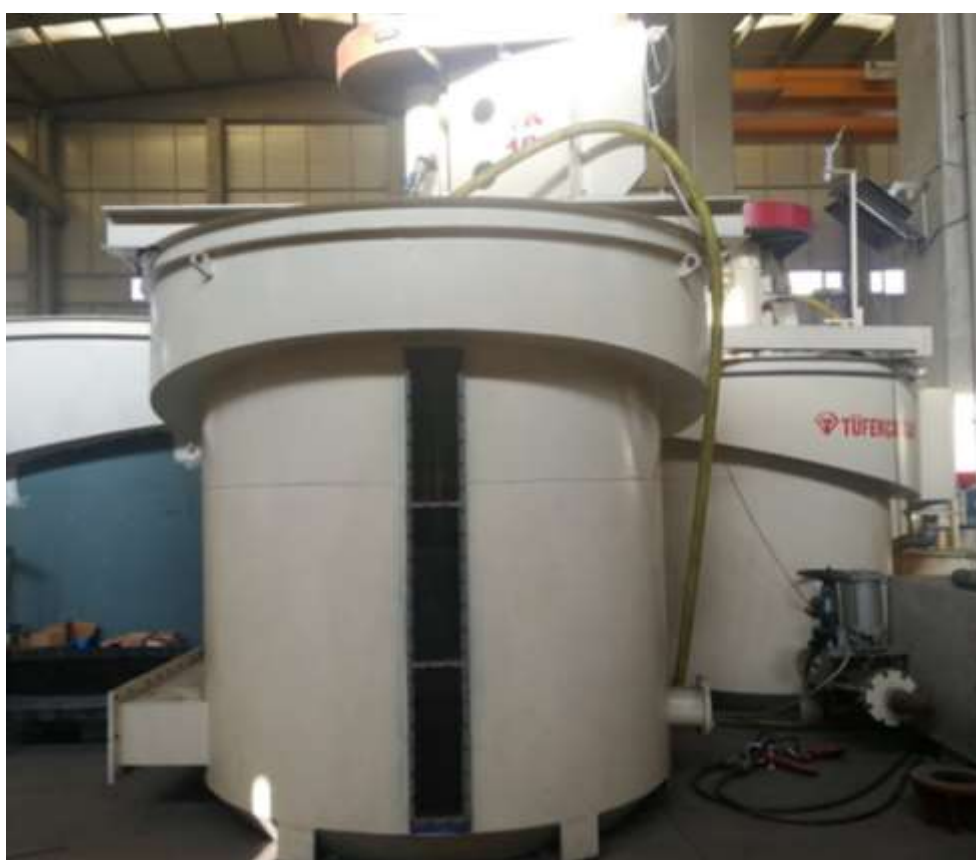
Figure 3. 10 m 3 Test Cell (Courtesy of Tüfekçioğlu)
