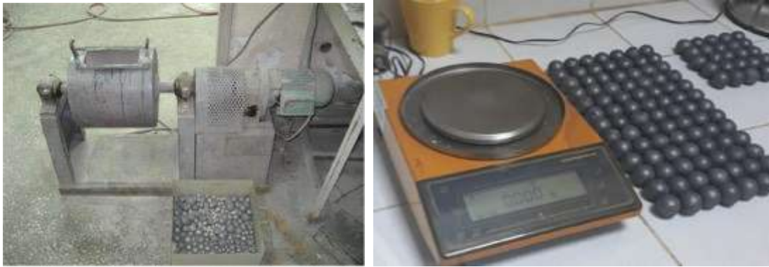
Figure 2. Laboratory scale ball mill & Weighing of the grinding medias
