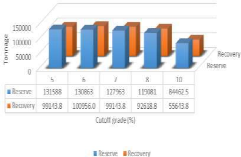
Figure 4. The effect of varying cutoff grade of zinc to minable reserve and recovery
