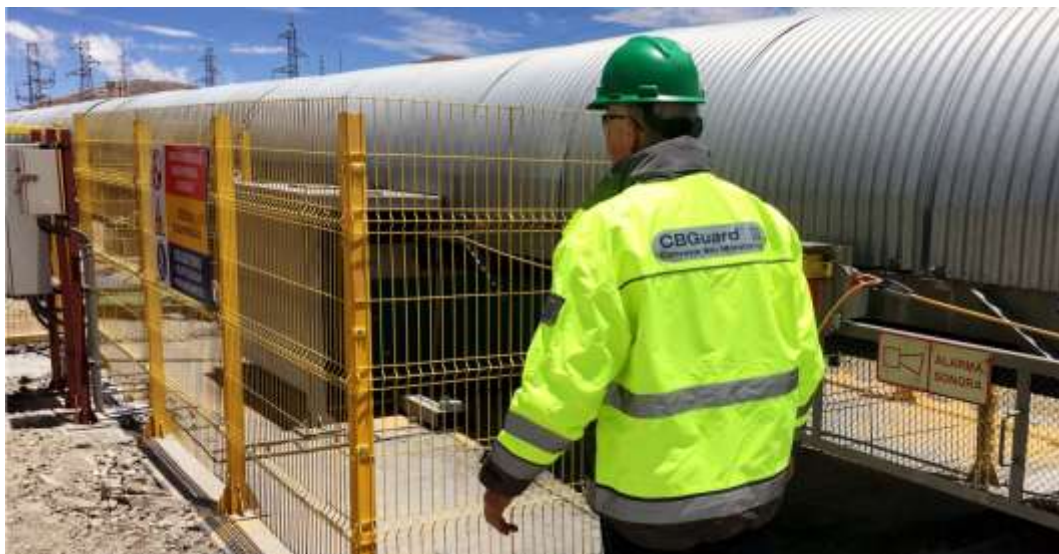
Figure 4. A CBGuard scanner with a safety fence in a copper mine
