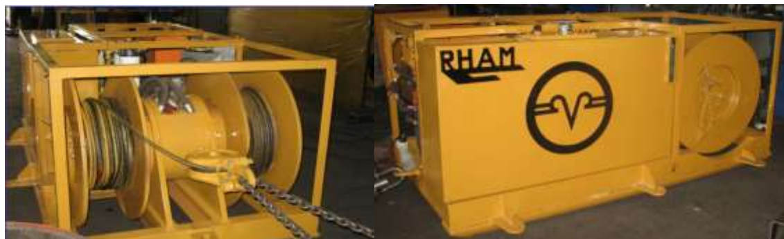
Figure 3. Rham hydrostatic remote control winch
