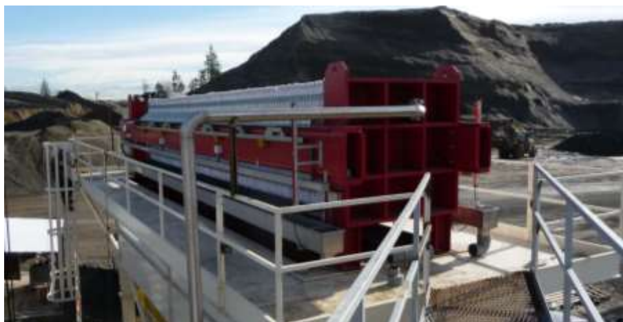
Figure 8. MATEC Filter Press Terra 1500/100PLT TT2 Fast plant, Pheonix, Poland
