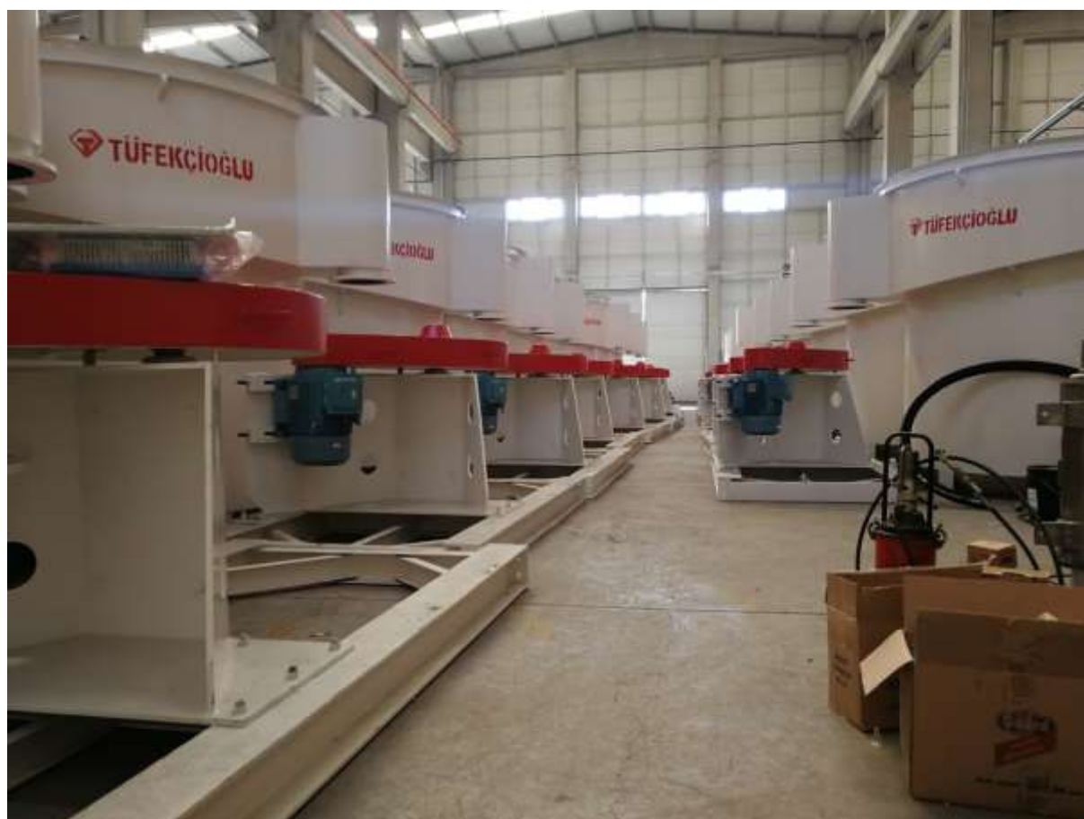
Figure 5. TK Cells Manufacturing in the Workshop (Courtesy of Tüfekçiöğlü).
