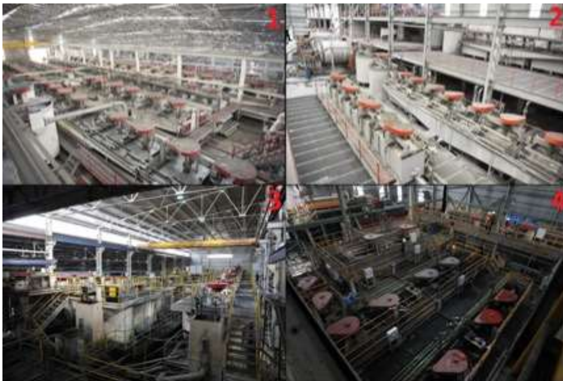
Figure7. Plants designed in house and machinery and equipment manufactured locally. (1) Balya (Pb-Zn 5000 tpd), (2) Ayazmant (Fe-Cu 900 tpd), (3) Gümüşhane (Pb-Zn-Cu 2000 tpd), (4) EtiBakır Samsun (Cu Slag 1700 tpd).
