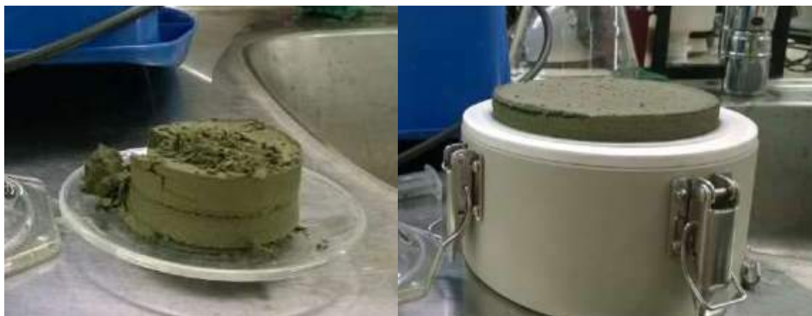
Figure 7. On the left: Cake with a residual moisture of 6.5 % wt by means of pressure filtration On the right: Cake from vacuum filtration test with a residual moisture of 15-17 % wt
