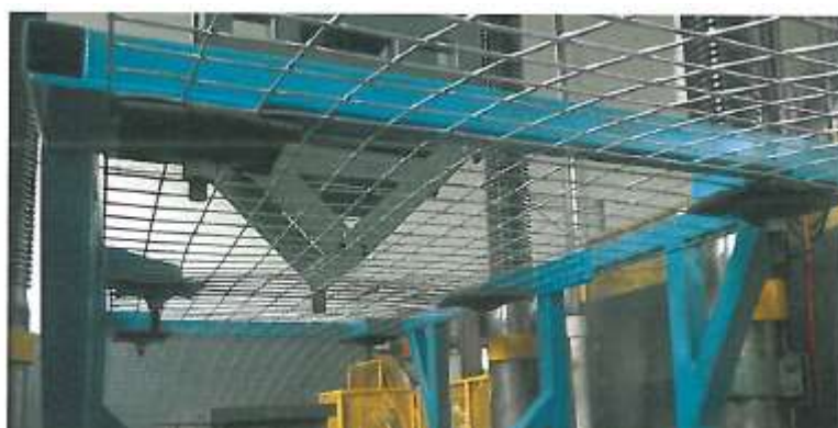
Figure 2. Dynamic test facility for surface support elements.
