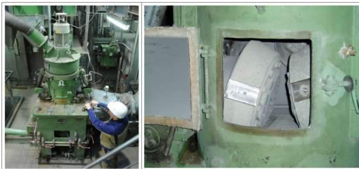
Figure 3. Test Centre lab mill and view into the grinding area
