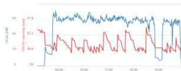
Figure 5. Power draw and CSS during a day of operation for a Hydrocone type crusher.
