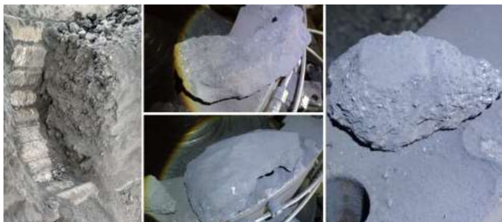
Figure 4 – Photographs of stratified particle-bed from inside eHPCC-2 concave liner
