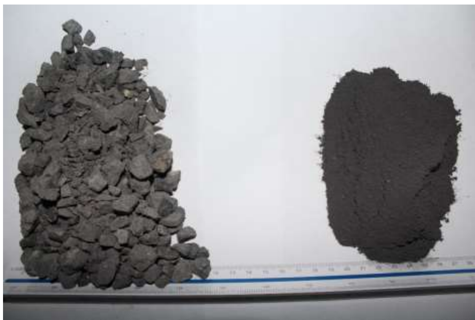
Figure 5. Magnetite concentrate – eHPCC-1 – feed and open-circuit product
