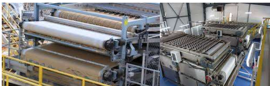
Figure 1. “Belt filter presses ( Kaswalder, 2018 )”
