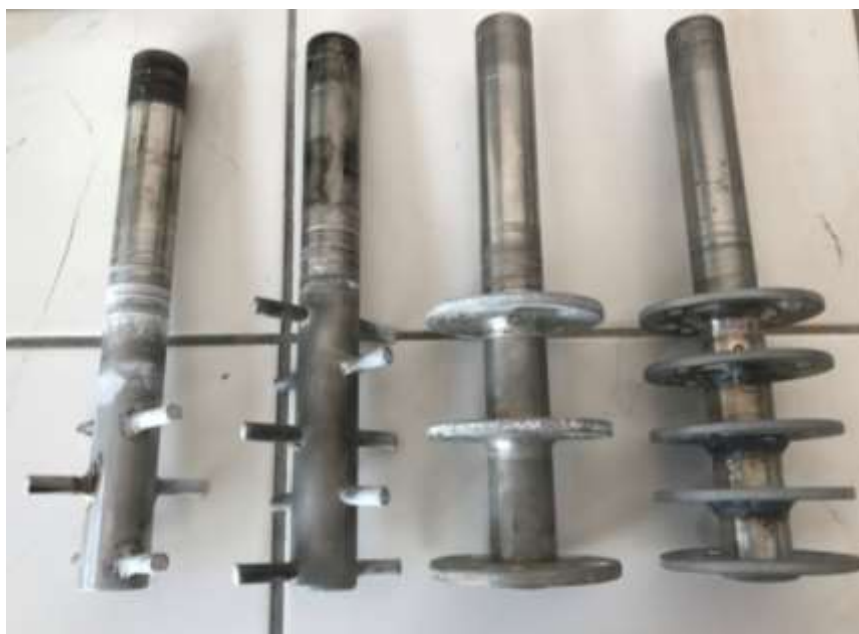
Figure 3. From left to right, three-pin, five-pin, three-disc and five-disc stirrer designs
