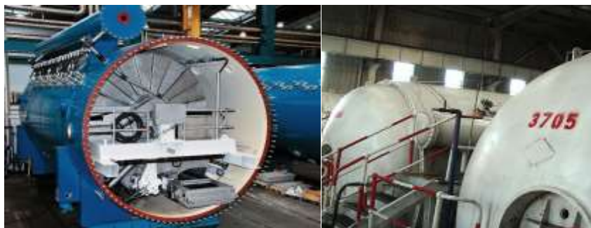
Figure 2. “Hyperbaric filters (Kaswalder, 2018)”
